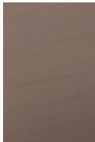
Ceiling - Lower Area Feature Wood Veneer on MDF Walnut finish Matte lacquer
